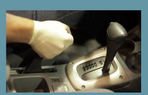
Place car in park, remove the keys and apply the parking
