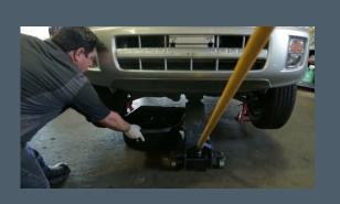
Place the oil recovery pan (drain pan) underneath the engine.
