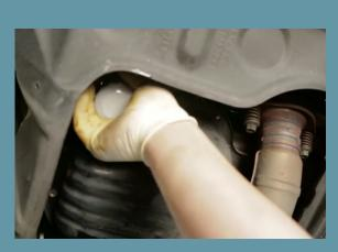
Carefully screw on the new, lubricated filter, being careful to not cross the threads.
